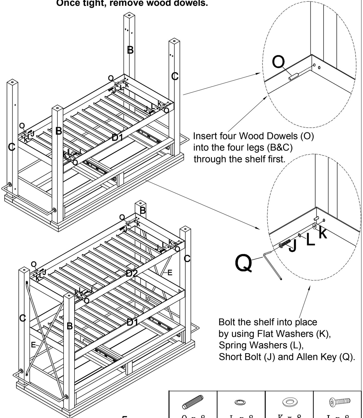
**Step 6.** Attach Rod (E) to Legs (B&C), using short Bolts (J) and Allen Key (Q) .
