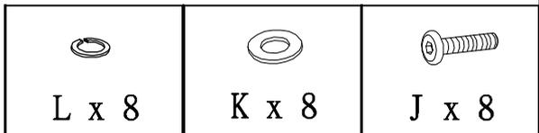
**Step 5.** Align Shelf (D1) with Legs (B&C) as shown below. Insert four wood dowels through the outer holes in the shelf (D1) into the Legs (B&C) to help hold the shelf in place. Install Flat Washers (K), Spring Washers (L) and Short Bolt (J) through the inner holes in the shelf into the Legs (B&C). Tighten with Allen Key (Q).
